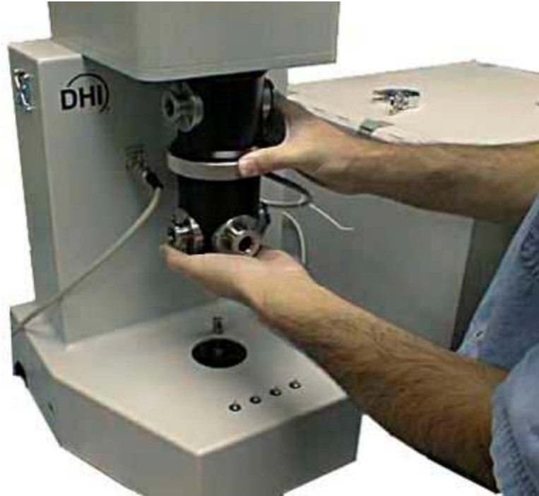
Figure 47. Removing the FPG8601 mounting post
