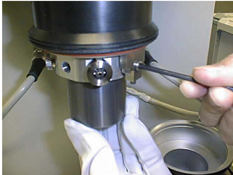
Figure 48. Removing the FPG8601 piston-cylinder
